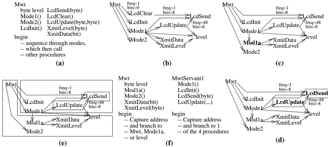
**Fig. 1:** The three partitioning steps on a simple example: (a) input specification with numerous procedures, (b) access graph, (c) granularity selection (using exlining), (d) pre-clustering, (e) N-way assignment (among 2 parts).
