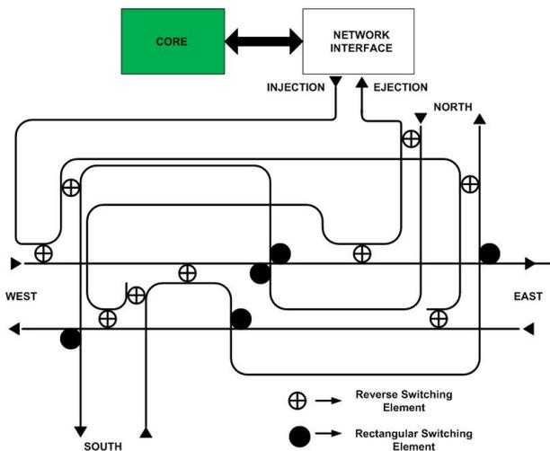
Fig. 3: Logical layout of MRRs in Photonic Router
