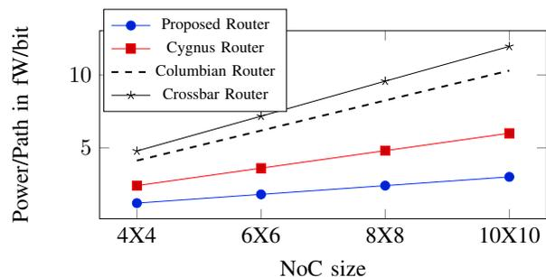
Fig. 9: Average Power/Path in fW/bit for different NoC sizes
