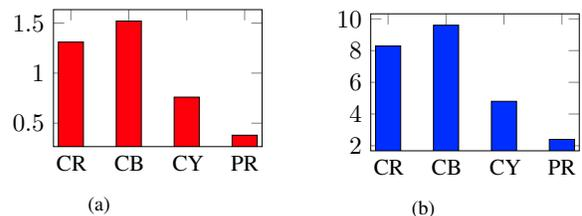
Fig. 8: (CR=Columbian Router, CB=Crossbar Router, CY=Cygnus Router, PR=Proposed Router) (a) Average Power Consumption per router in fW/bit (b) Average Power Consumption per optical path of  $4 \times 4$  photonic mesh in fW/bit
