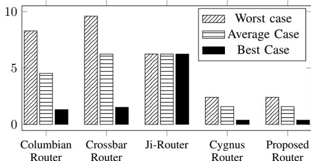
Fig. 10: Insertion loss per router in dB
