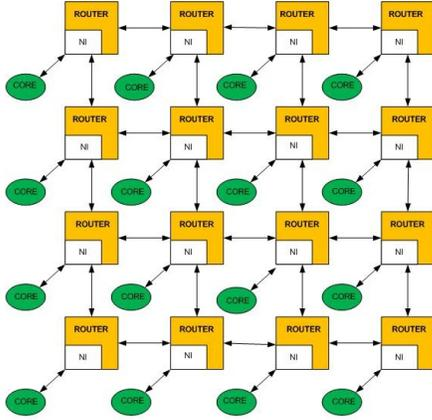
Fig. 1: Two Dimensional Photonic mesh network
