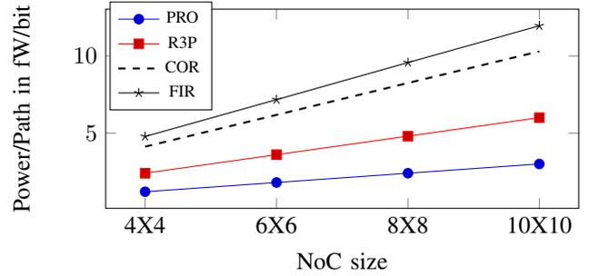
Fig. 7: Average power per Path for different NoC sizes
