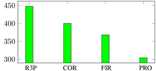
Fig. 5: Comparing number of MRRs for  $4 \times 4$  PNoC; R3P:R-3PO, COR:Corona, FIR:Firefly, PRO:proposed 2-layer PNoC
