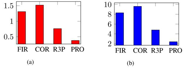
Fig. 6: Comparison of power consumption (a) per router and (b) optical path, in fW/bit
