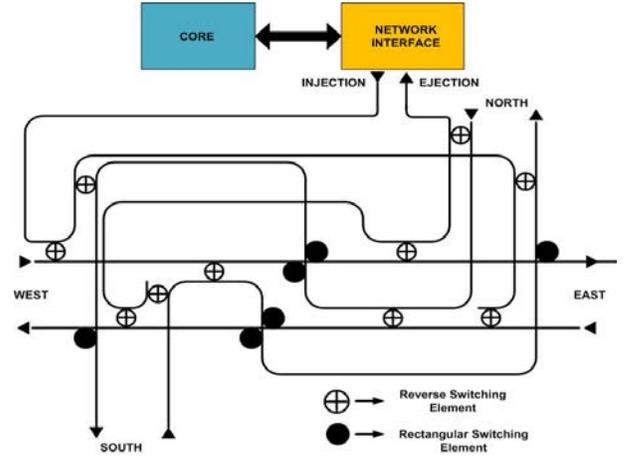
Fig. 3: Logical layout of  $5 \times 5$  photonic router
